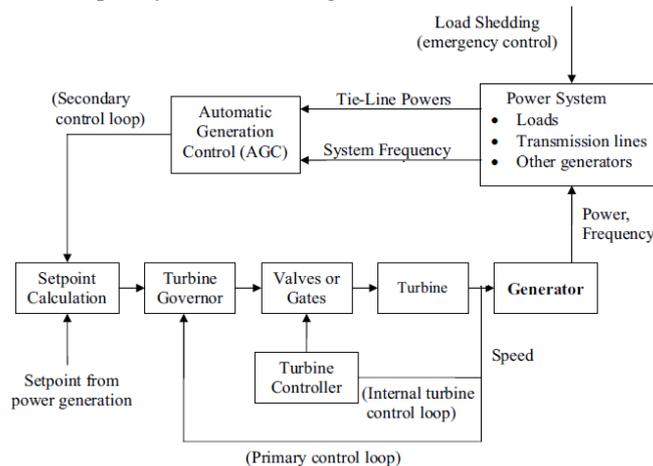
Figure 4. Control Structure for frequency control system
