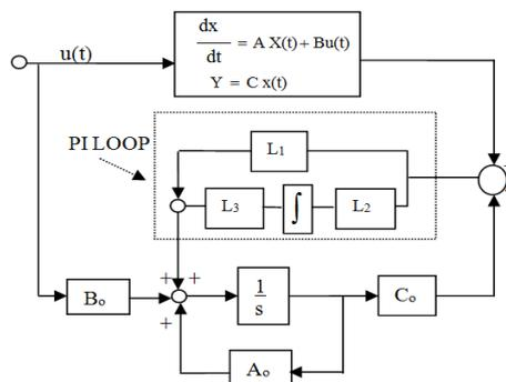
**Figure 3.** Block diagram of PI-observer
